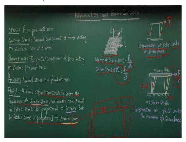
You as know it when you apply a force then you will have a stress concentrations on that. For example as is given here there is a surface in which we have applied the force component which has a tangential component also the normal component. Because of this normal component, you will have the normal stress components acting on that. Then you will have the shear stress component on that.
