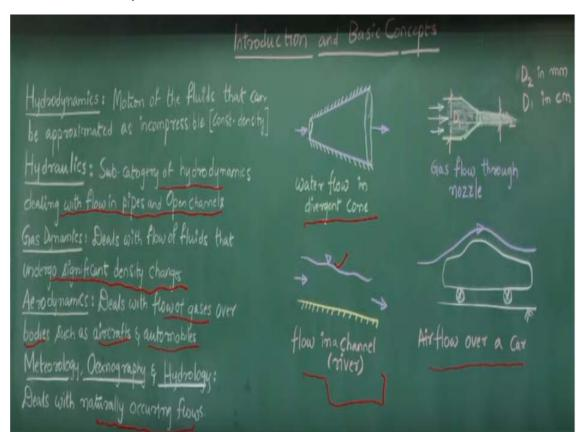
Considering that let us go to we also classified the problems the based on a different conditions like the compressibility, like the fluid properties that is what one of the basic properties is fluid density, the mass per unit volume. If it is the density changes, then we call it fluid is compressible. If density does not change then we call fluid is incompressible.
