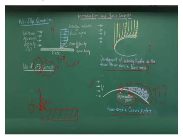
Let have talk about a very interesting concept which is called no-slip conditions. When a fluid flow through a having a interface with a solid surface, what is the conditions prevails it. For examples, if I have the plate, which is at the rest conditions the velocity is zero and I have the uniform flow is coming from the left side. As the fluid flow touches over that of the surface is the condition is called is no-slip conditions.
