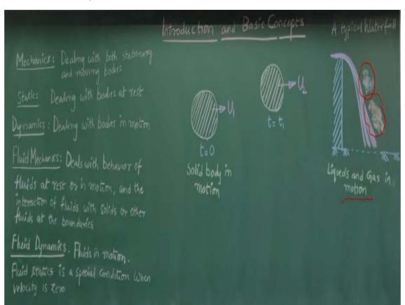
Now let us talk about the introductions and the basic concept. As you know it when you talk about the mechanics we talk about the flow of dealing with the both stationary and the moving object. So like for examples what is given here you can have a solid body is translation rotation, the rotation position can have a shear stress, shear strain all you know it in solid mechanics.
